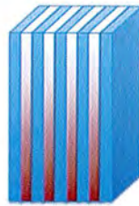
Bullet proof glass consisting of normal glass (blue) and polycarbonate (red) layers
